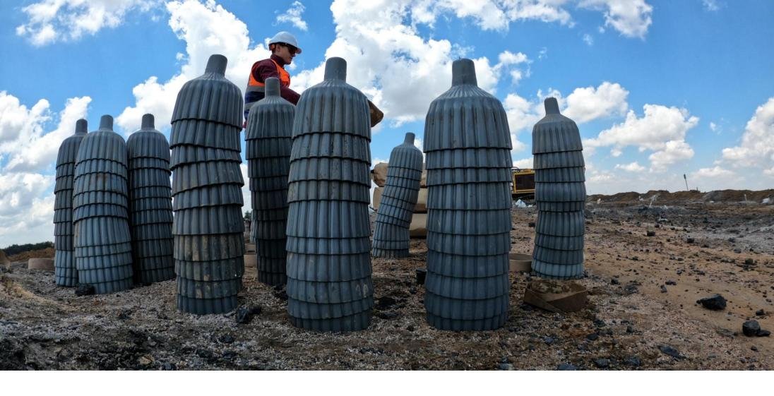
WE DID THIS BY FOCUSING ON IMPROVED ENERGY RETENTION AND DISTRIBUTION DURING BLASTING, USING VARISTEM® STEMMING PLUGS AS THE KEY TOOL TO EFFECT THIS CHANGE
